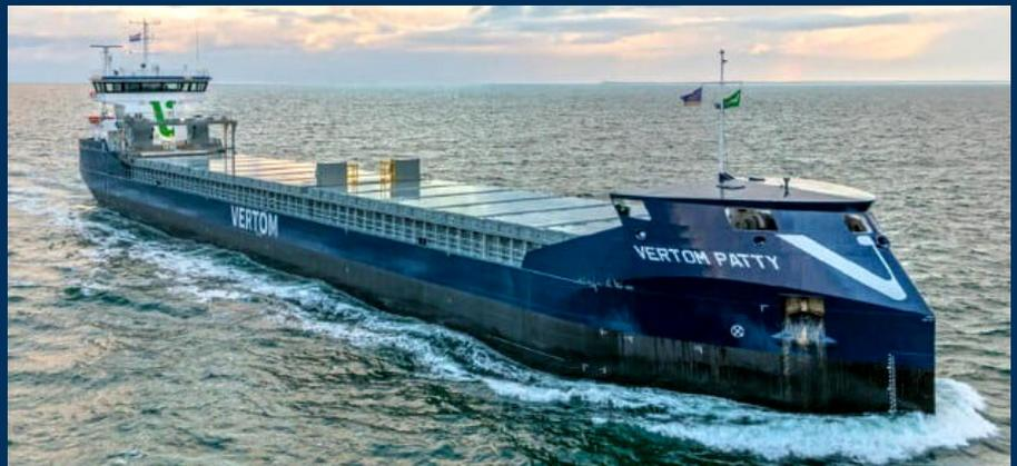
The LABRAX design was developed to Vertom's requirements and to provide both a highly efficient ship as well as one with versatility in its cargo operations. The completely box-shaped cargo holds ensure optimal loading flexibility and maximum cargo intake. The vessel is capable of grain or bale loading and
